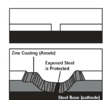
This is what happens to a scratch on galvanized steel. The zinc coating sacrifices itself slowly by galvanic action to protect the base steel. This sacrificial action continues as long as any zinc remains in the immediate area.
